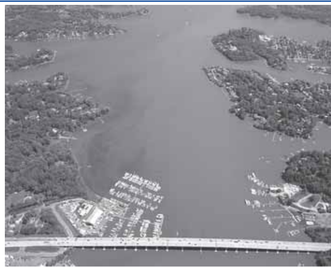
Figure 1. The South River After a 3.3-inch Rain Event (two-year storm) in May 2008.
